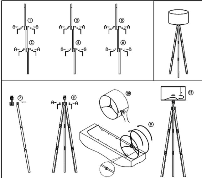
A. Step1-6:Jabbing and screwing bits in place,secure with the provided hexagon wrench.
