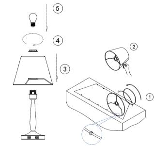
① ② Place the two rollers on the lampshade in the same direction as shown in the figure, and press them on the plastic buckle to make them completely coincide, pay attention to the inner installation of the roller protruding part towards the lampshade.
