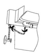
To assemble the braided hose to the water inlet end of bidet and turn tight.
