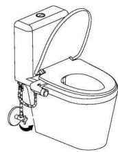
Adjust the knob according to the picture showing, turn on the angle valve, and then check if any leaking happening in each connector.
